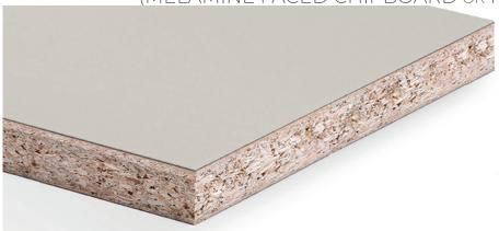
Chipboard is composed of wood particles (core of the brown board), covered with a decorative paper impregnated with melamine resin
