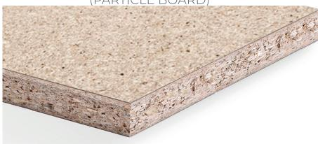
Chipboard is also known as a practice board. This type of board is made by mixing wood particles with resin and with heat and pressure applied during manufacture a rigid board is created.
