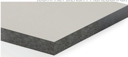
High-density Kraft fiber board, mass dyed in black, core of the board in black, white, brown or sandwich (fiber), covered with two layers of barrier paper (brown or white) and a decorative paper impregnated with melamine or phenolic resin, on each side, resulting in a multilayer composition.
