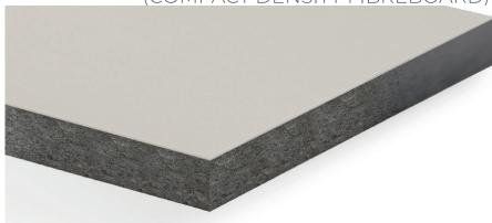
High-density resistance compact board, formed by a core of sheets of Kraft paper (grey or white core) and a decorative paper on one side, all impregnated with melamine resin.
